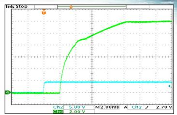
Figure 8: Turn-on transient at full resistive load and 5mF output capacitance initiated by ENA1. Input voltage pre-applied. Ch 2: ENA1 (5V/div). Ch 4: Vout (2V/div). Timebase: (2ms/div).
