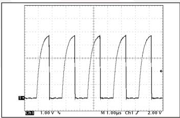
Figure 17: SYNC OUT vs. time, driving SYNC IN of a second SynQor MQHL converter. Ch1: SYNC OUT: (1V/div). Timebase: (1us/div).
