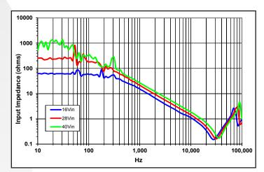
Figure 21: Magnitude of incremental input impedance (Zin = vin/in) for minimum, nominal, and maximum input voltage at full rated power.
