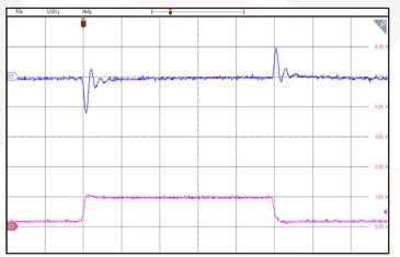
Figure 11: Output voltage response to step-change in load current 0%-50%-0% of Iout (max). Load cap:  $1\mu F$  ceramic cap and  $10\mu F$ ,  $100m\Omega$  ESR tantalum cap. Ch 1: Vout (200mV/div). Ch 2: Iout (1A/div). Timebase: (400 us/div)
