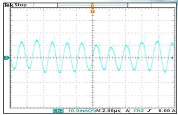
Figure 14: Input terminal current ripple, ic, at full rated output current and nominal input voltage with SynQor MQ filter module (10mA/div). Bandwidth: 20MHz. Timebase: (2us/div). See Figure 13.
