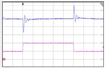
Figure 10: Output voltage response to step-change in load current 50%-100%-50% of lout (max). Load cap: 1μF ceramic cap and 10μF, 100mΩ ESR tantalum cap. Ch 1: Vout (200mV/div). Ch 2: Iout (1A/div). Timebase: (400 us/div)
