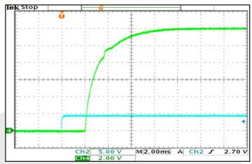
Figure 7: Turn-on transient at full resistive load and zero output capacitance initiated by ENA1. Input voltage pre-applied. Ch 2: ENA1 (5V/div). Ch4: Vout (2V/div). Timebase: (2ms/div).
