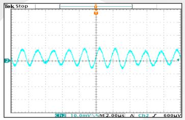
Figure 15: Output voltage ripple, Vout, at nominal input voltage and rated load current (10mV/div). Load capacitance:  $1\mu F$  ceramic capacitor and  $10\mu F$  tantalum capacitor. Bandwidth: 20MHz. Timebase: (2us/div). See Figure 13.
