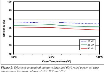
temperature for input voltage of 16V, 28V, and 40V.
