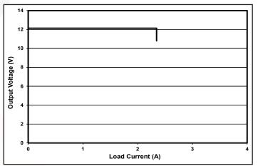
Figure 6: Output voltage vs. load current showing typical current limit curves at
