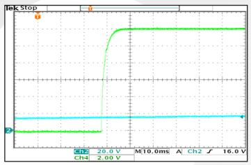
Figure 9: Turn-on transient at full resistive load and zero output capacitance initiated by Vin. ENA1 previously high. Ch 2: Vin (20V/div). Ch 4: Vout (2V/div). Timebase: (10ms/div).
